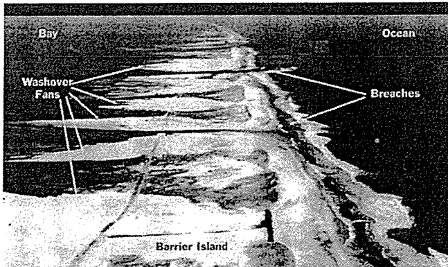
Figure 9. Washover fans and breaches caused by the 1938 hurricane in the Westhampton area. (Photo: U.S. Army Corps of Engineers 1958)
